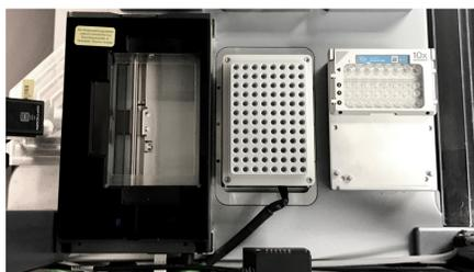
Figure 1. The layout for automated chip loading, from sample 2D barcode tube scan, to a barcoded chilled PCR plate, to 10X chip.
